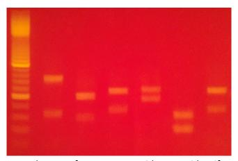
In a crime scene, DNA samples are often a strong evidence to identify a particular individual. These DNA samples are analyzed by DNA electrophoresis. In the Forensic DNA Gel Electrophoresis Kit, there are DNA samples found in a virtual crime scene and from 5 suspects. By comparing the DNA bands of different samples, students can act as detectives to find out which suspect is the most suspicious!
